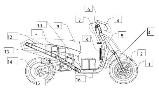
Fig. 1: Hybrid scooter parts
